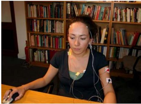
Two electrodes are placed on the left side chest above and below the heart to provide an electrocardiogram (ECG). The two on the left arm measure muscle tension while the electrodes on the scalp measure the small amounts and frequencies of electrical energy generated by the brain (EEG). The silver ear clips act as reference points.
