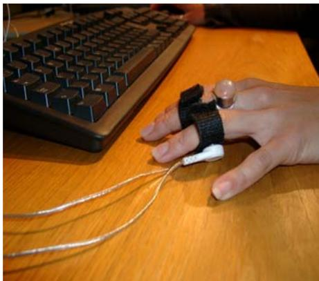
The box to which these wires lead is a 'MindPeak WaveRider', shown in Figure 3. The computer, to which the box in turn is connected, can be programmed to emit musical tones as the various measures of heart, muscle, brain etc. rise and fall. By using the feedback this 'music' provides, you can make yourself relax by 'thinking' your heart rate and muscle tension down.
